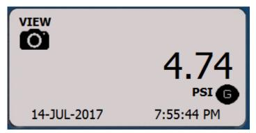
The date and time is stored with each snapshot. Any new snapshots taken will overwrite the oldest stored in memory.
