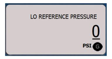
Certain pressure ranges may have more than two pressure reference setpoints. Follow the same procedure of entering in the known value and confirming with SELECT key. Once the calibration is complete verify the gauge is within specification by the running the up and down scale throughout range. Reference the original Certificate of Calibration for cardinal points.
