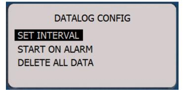
Datalogging can be setup to automatically start on an Alarm condition as well. Simply choose START ON ALARM and press SELECT. Datalogging will start based on either the High or Low alarm setting and run at the defined interval from that point forward. Clearing the alarm will not turn off Datalogging.
