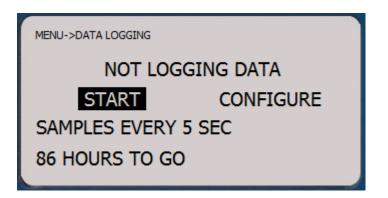
To change settings select CONFIGURE. The sample rate can be set from 1 second to 24 hours. Just use the arrows key to desired value and press SELECT to confirm.
