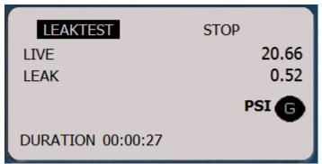
To stop the test at any time press right arrow to highlight STOP. When the test is complete, the gauge will display the leak rate in units/minute. In addition, the results with start time and end time are displayed until the next test is started. Minimum test time is 10 seconds. To start a new test use the left arrow key.
