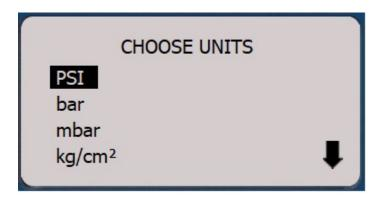
Press the UNITS key to accept the selection and the gauge will return to *Measure Mode*.
